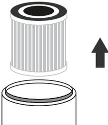
3. Clean out any remaining dust or hair inside the purifier using a vacuum hose. Do not use water or liquids to clean the purifier. Unwrap the new air filter and place it into the housing.
